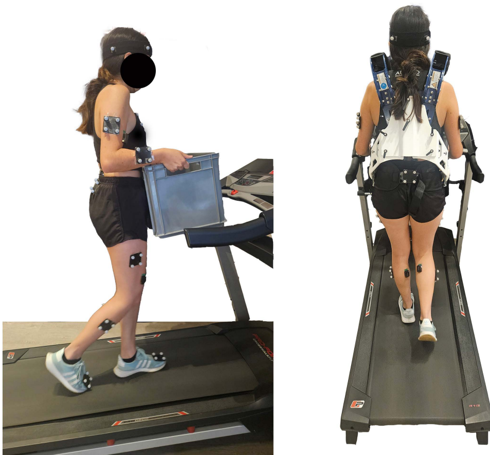
Fig 1. Participant wearing the CarrySuit® exoskeleton and walking on a treadmill with the highest inclination.
